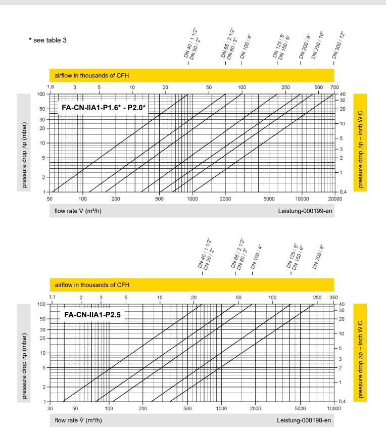
The flow capacity charts have been determined with a calibrated and TÜV certified flow capacity test rig. Volume flow  $\dot{V}$  in (m³/h) and CFH refer to the standard reference conditions of air in ISO 6358 (20°C, 1bar). For conversion to other densities and temperatures, refer to Sec. 1: "Technical Fundamentals."
