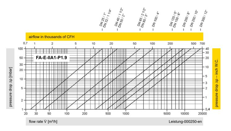
The flow capacity charts have been determined with a calibrated and TÜV certified flow capacity test rig. Volume flow  $\dot{V}$  in (m<sup>3</sup>/h) and CFH refer to the standard reference conditions of air in ISO 6358 (20°C, 1bar). For conversion to other densities and temperatures, refer to Sec. 1: "Technical Fundamentals."
