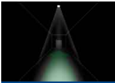
Escape route illumination with asymmetric optics.
