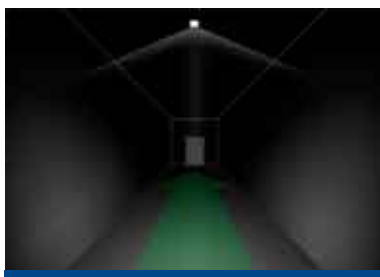
Escape route illumination with symmetric optics.
